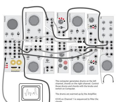
Notes from Channel 2 go the oscillator and gates trigger the slopes, which controls the second filter to make basslines or a lead line.
